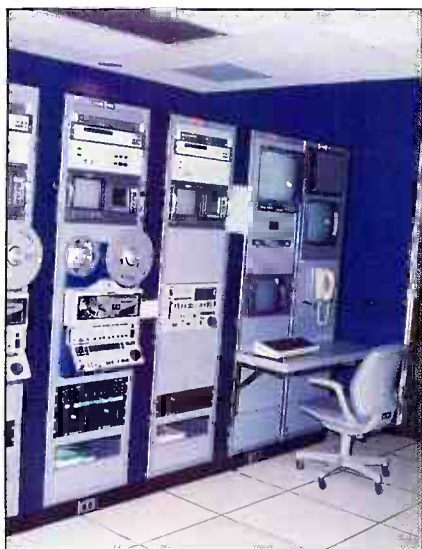
The SAM terminal (at the far right) is used by the videotape operator to access the automation system for informational purposes. No changes in the air schedule can be made from this terminal.
